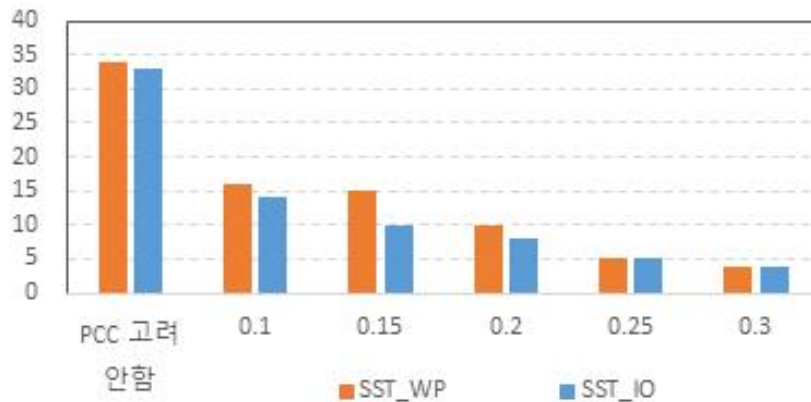
Figure 58. Total number of cases of SST_WP (orange bar) and SST_IO (blue bar) without considering PCC (N_total; first column) and with considering PCC (N_PCC_total; from second to 6th column). When considering PCC, values of PCC (Threshold_PCC) vary from 0.1 to 0.3. Among HGT200, HGT850, and OMG500, if PCCs are greater than Treshold_PCC for more than two variables, it is considered to be a hit.
