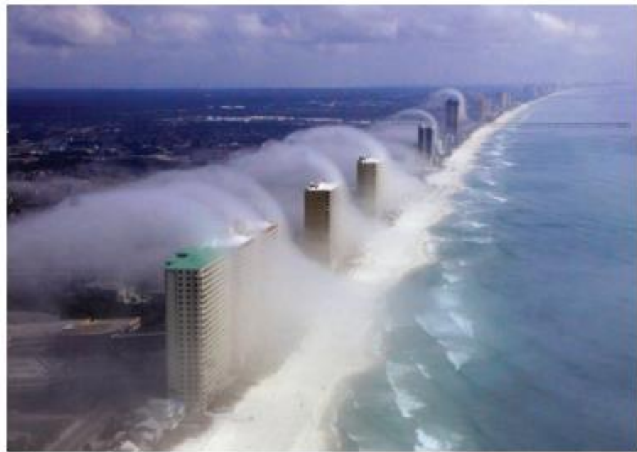
Figure 4.7 Clouds that visualize flow displacement over high-rise buildings in Panama City Beach, United States. Wind is from the ocean (Credit: J. R. Hott, Panhandle Helicopters; with permission).
