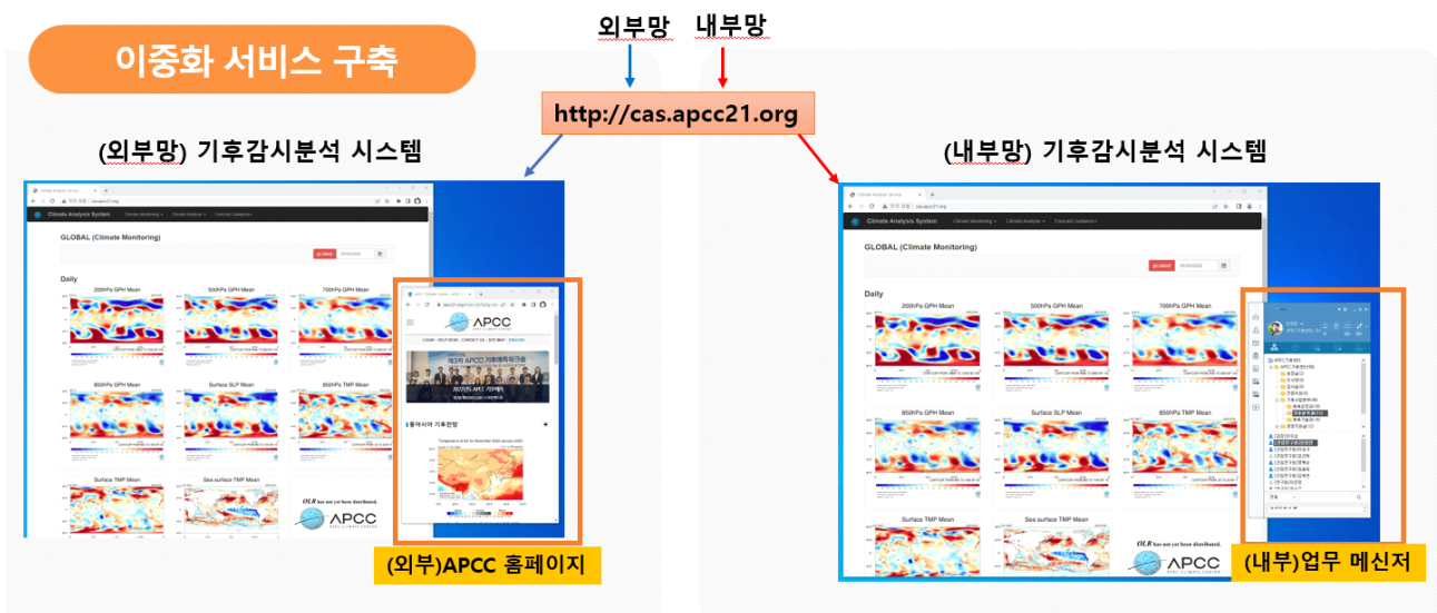
Figure 126. A dual service was built so that users can the same climate analysis system even when accessing from the internal or external Internet network.
