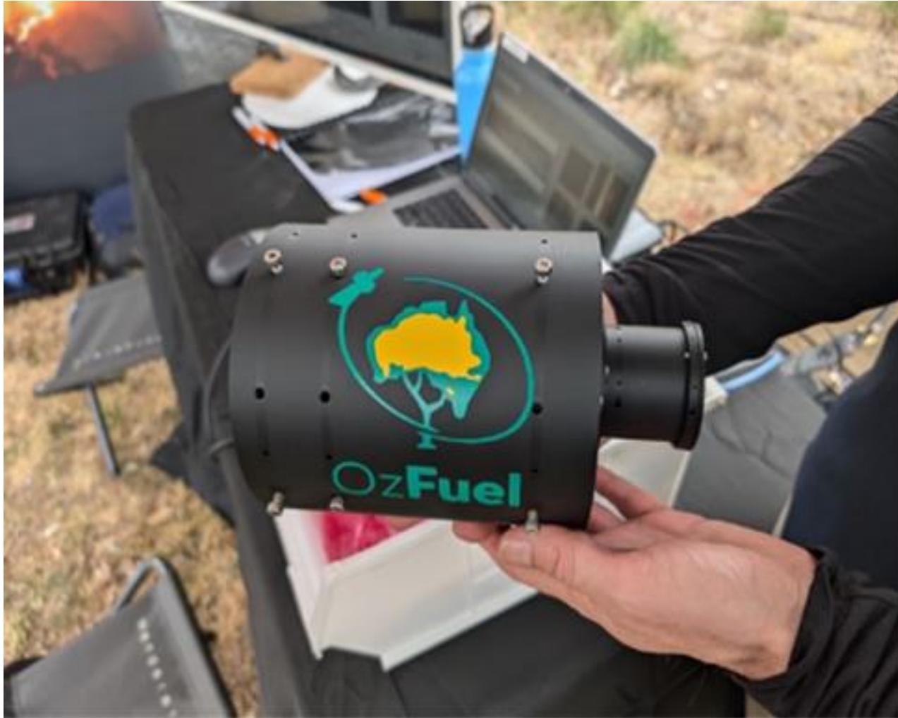
ANU 3D printed engineering model for the OzFuel telescope
