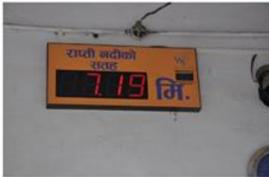
Display board at DAO, Banke showing water level of Rapti River at Kusum (above danger level)
